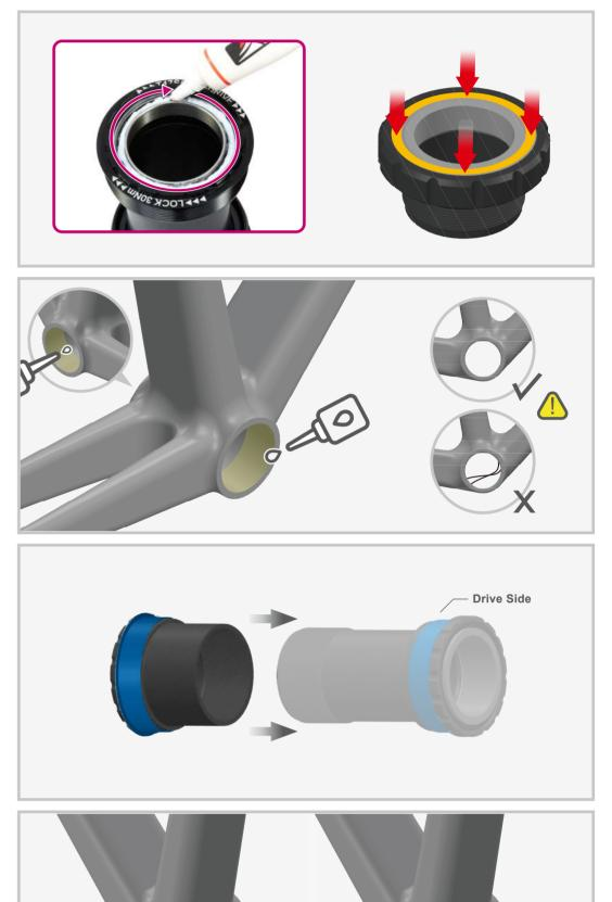
A During pressing, ensure the BB is inserted at a proper vertical angle to the frame. If you encounter excessive resistance while pressing, stop the process and recheck the insertion angle and the BB shell for any debris or deformation.
